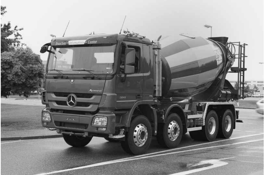
Figure 27.13 An eight-wheel rigid vehicle equipped with a cement hopper
