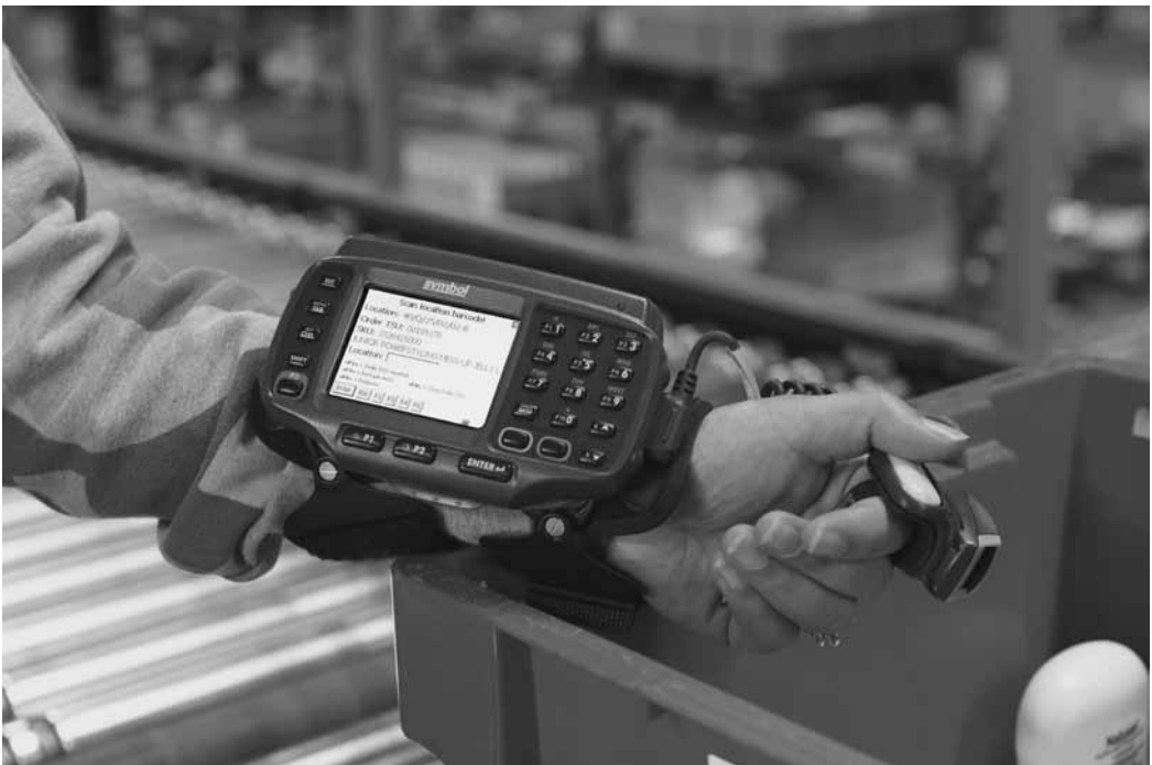
Figure 19.6 Wrist-mounted radio data terminal with ring bar-code scanner
