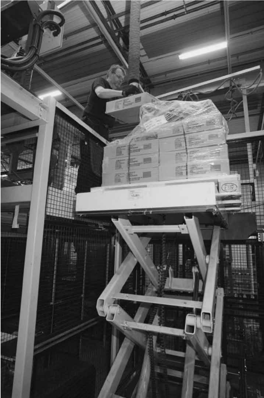
Figure 22.1 Scissor lift and suction handling equipment to aid manual handling activities
