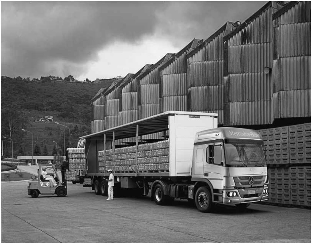
Figure 27.11 A curtain-sided trailer giving ease of access for loading
