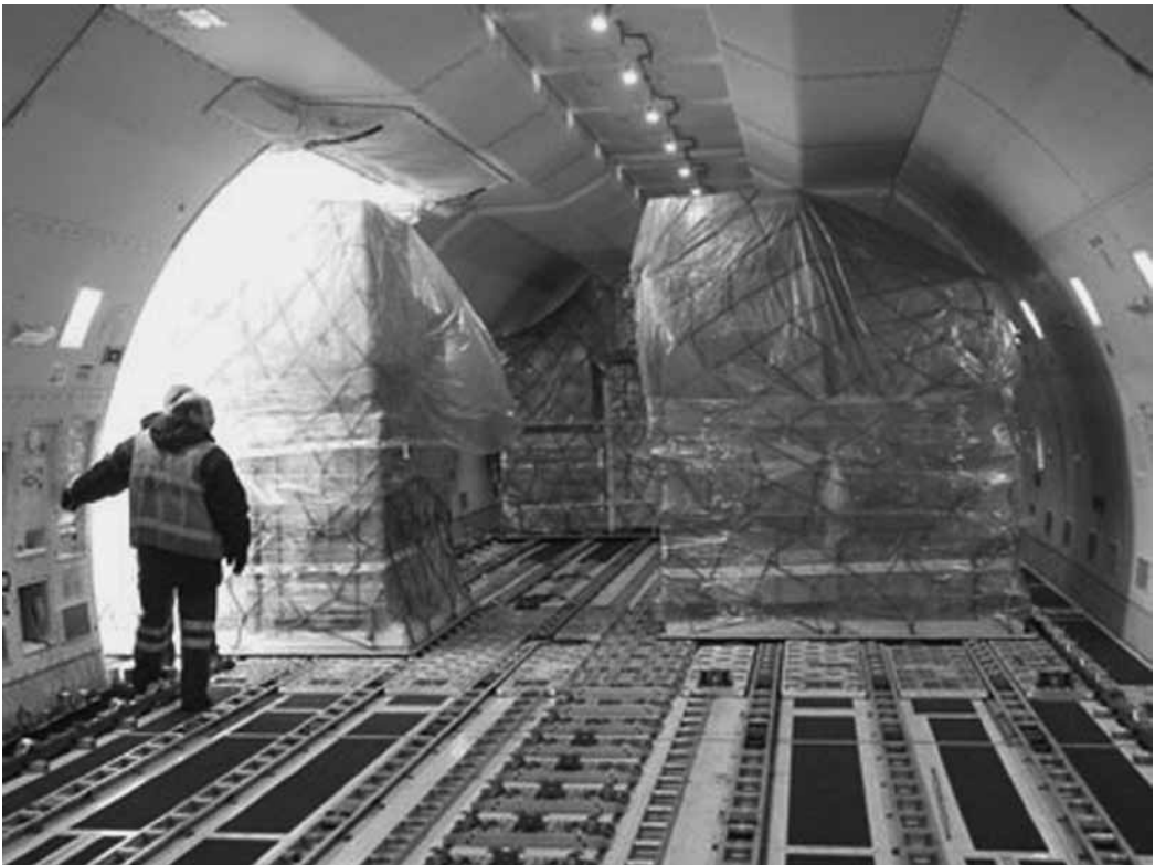
Figure 25.2 A Cargolux air freighter being loaded through the side door
