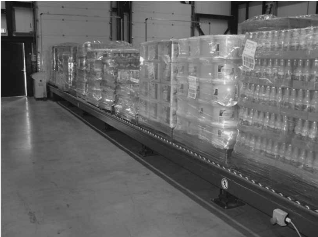
Figure 20.2 Pallets on a conveyor system, ready for automated loading/unloading
