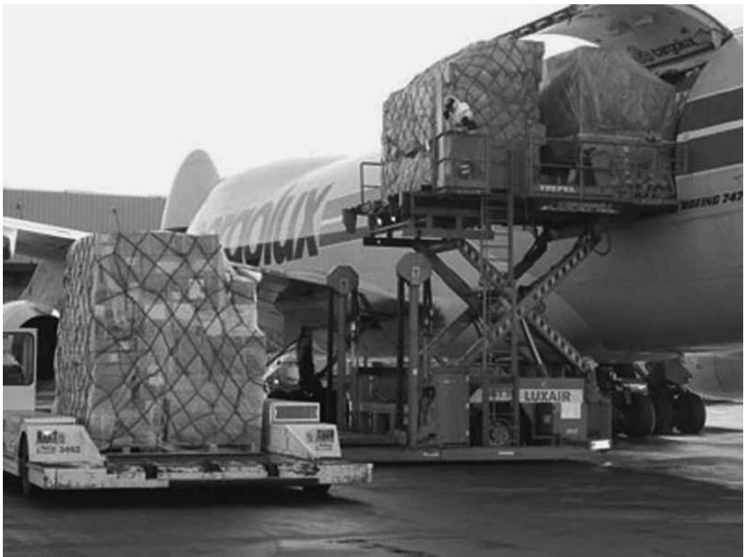
Figure 25.1 Air cargo pallets being loaded on to an air freighter
