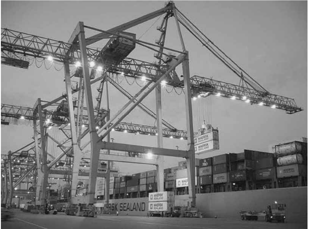
Figure 26.4 A ship to shore gantry crane loading a cellular container ship
