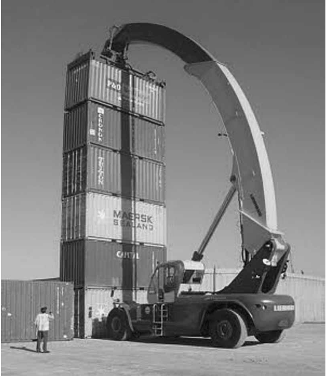
Figure 26.6 A reach stacker stacking ISO containers
