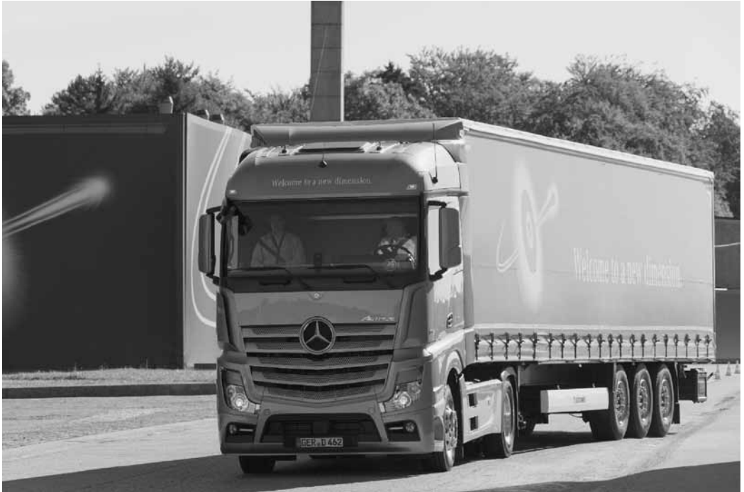
Figure 27.1 An articulated vehicle comprising a tractor and curtain-sided semi-trailer
