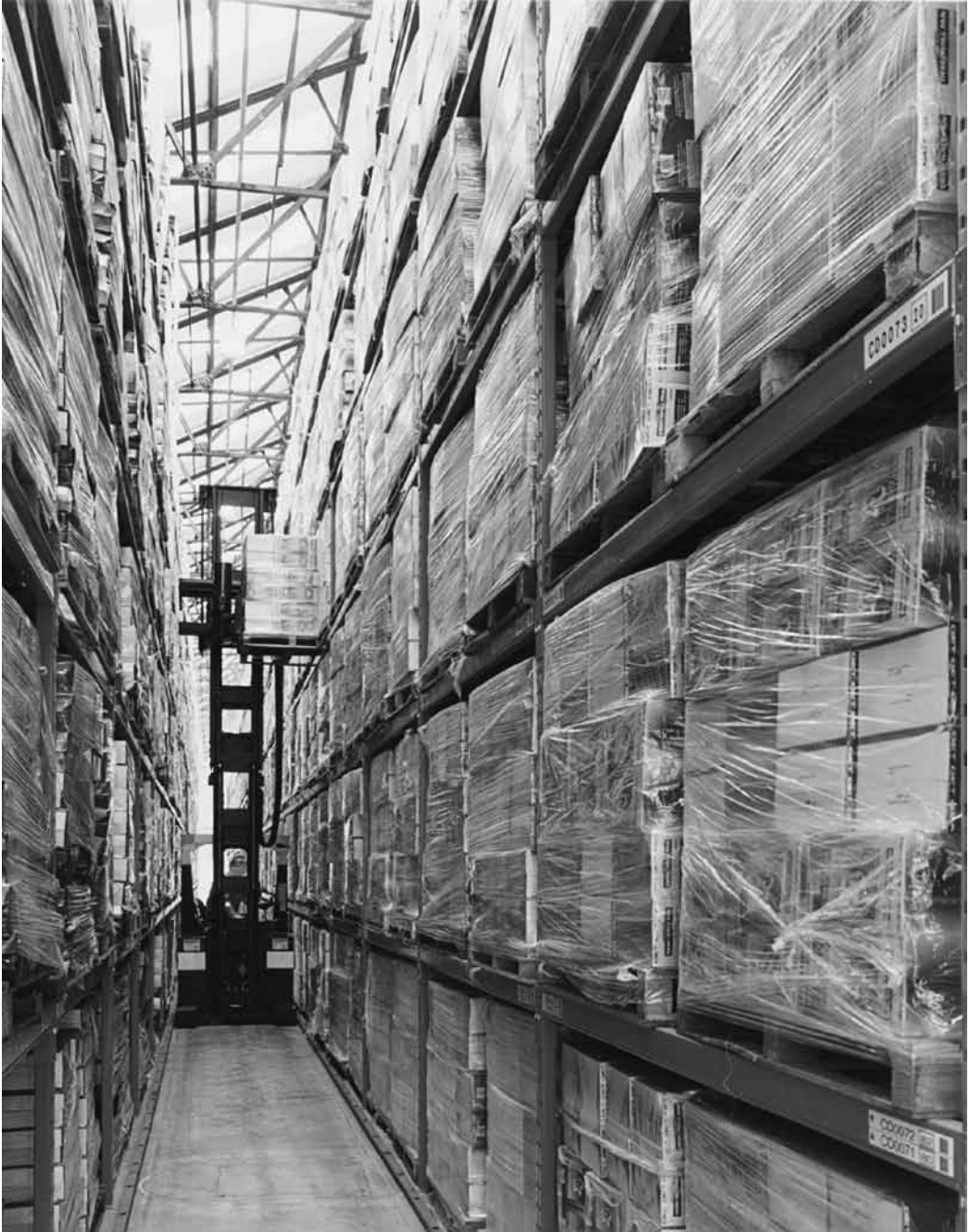
Figure 17.7 Narrow-aisle truck, positioning pallet in narrow-aisle racking
