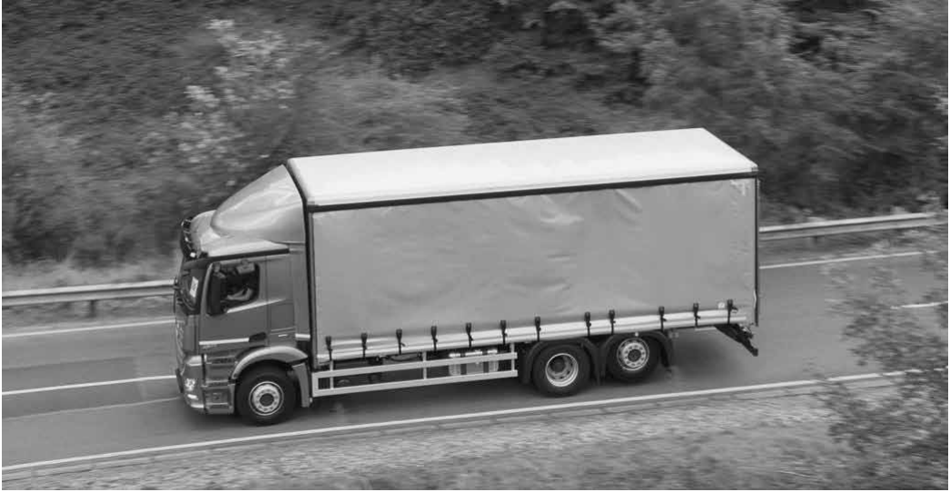
Figure 27.2 A six-wheeled rigid vehicle fitted with a lifting rear axle
