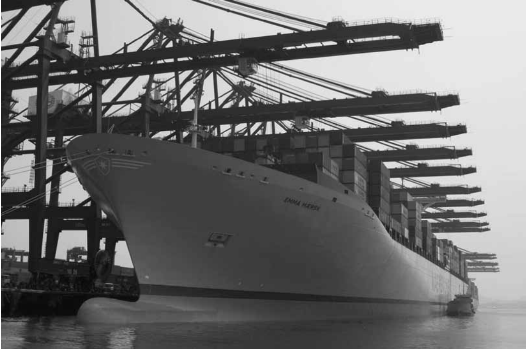
Figure 24.2 The Emma Maersk : the second largest cellular container vessel in the world, capable of transporting 15,200 TEU
