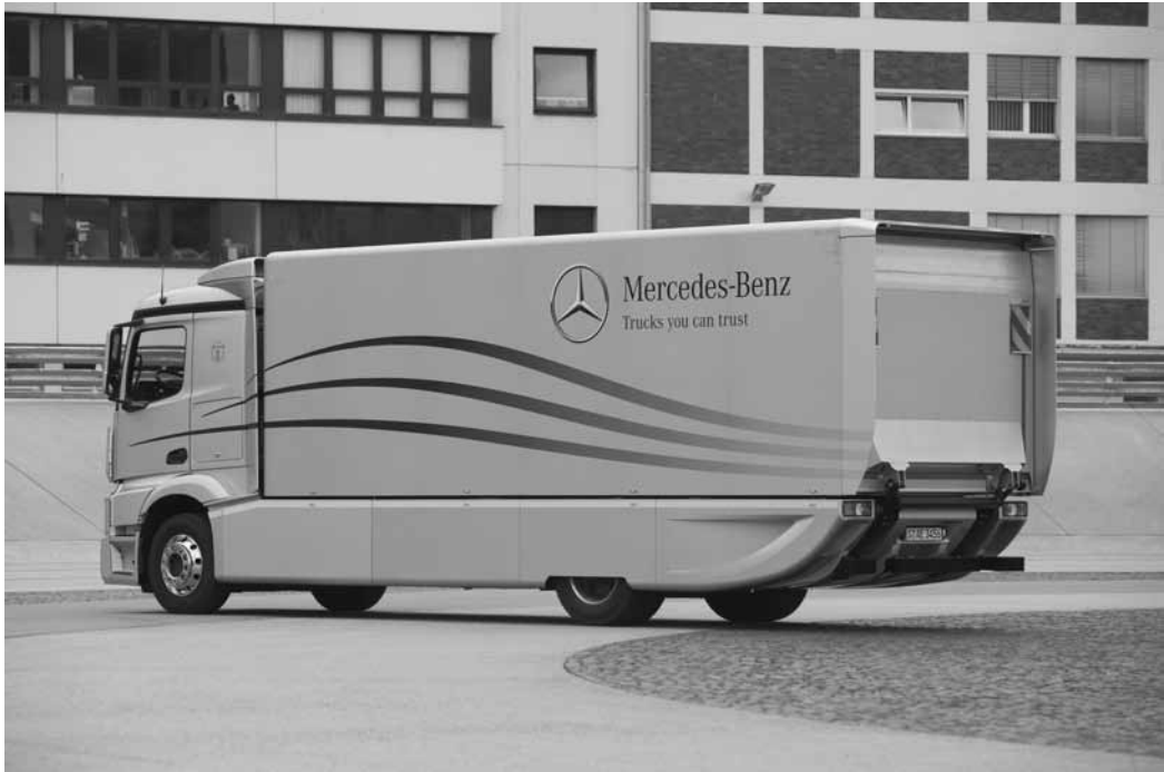
Figure 37.1 A rigid vehicle designed to be more aerodynamic
