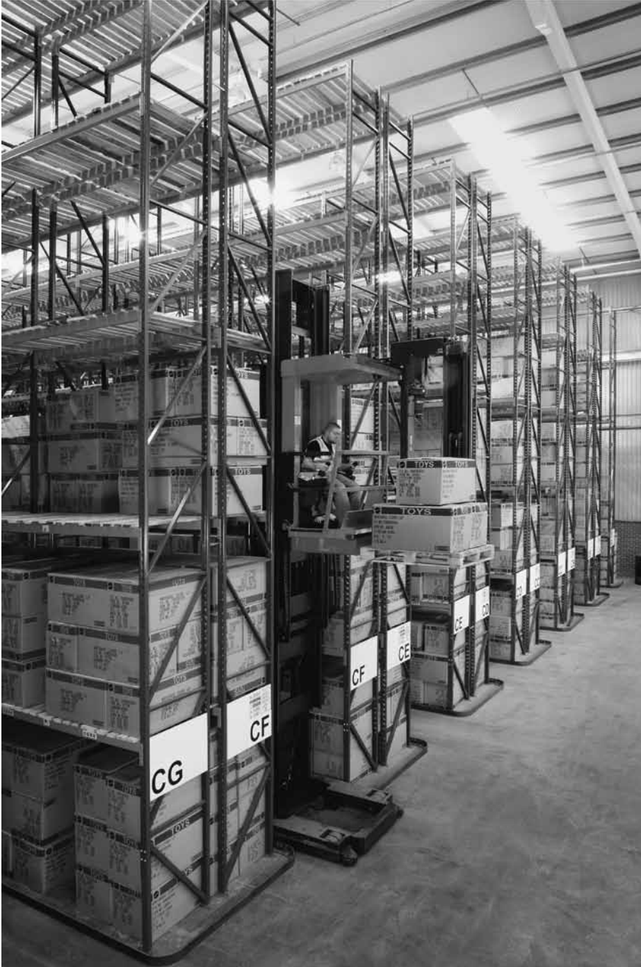
Figure 19.2 Free-path high-level order picking truck, operating in narrow aisle
