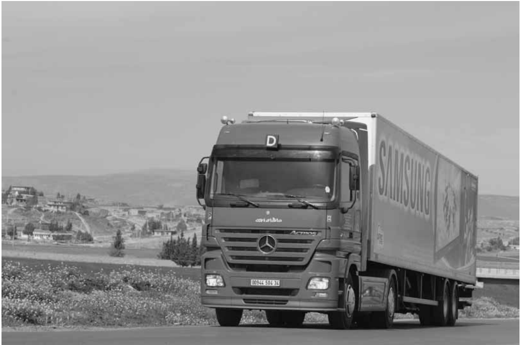
Figure 27.9 An articulated combination featuring a box trailer
