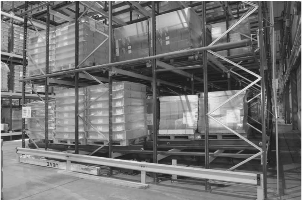
Figure 17.5 Five-deep push-back racking, also showing in-rack sprinklers for fire suppression and barriers to avoid damage collision to the rack uprights
