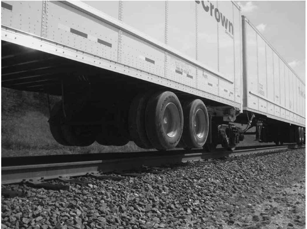
Figure 26.2 RoadRailer® semi-trailers coupled to form railway rolling stock
