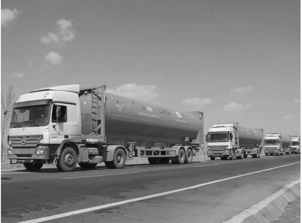
Figure 26.1 An articulated vehicle loaded with a tanktainer
