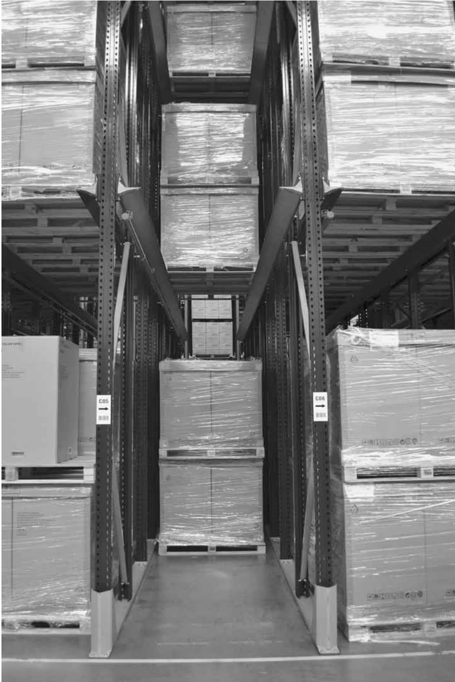
Figure 17.4 Drive-in racking, showing pairs of pallets being supported in the racking
