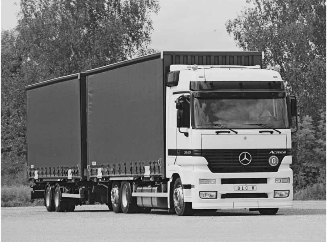
Figure 27.4 A high cubic capacity close-coupled draw-bar combination
