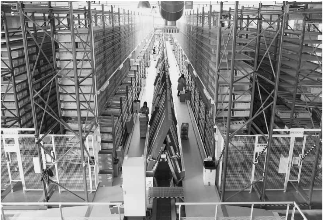
Figure 19.4 A-frame dispenser, showing the dispenser in the centre and low-level flow racks on either side holding items in tote bins ready for replenishment
