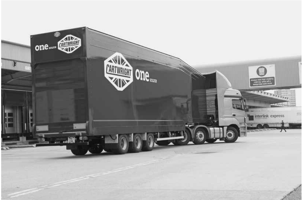
Figure 27.5 An articulated vehicle featuring a double-deck trailer
