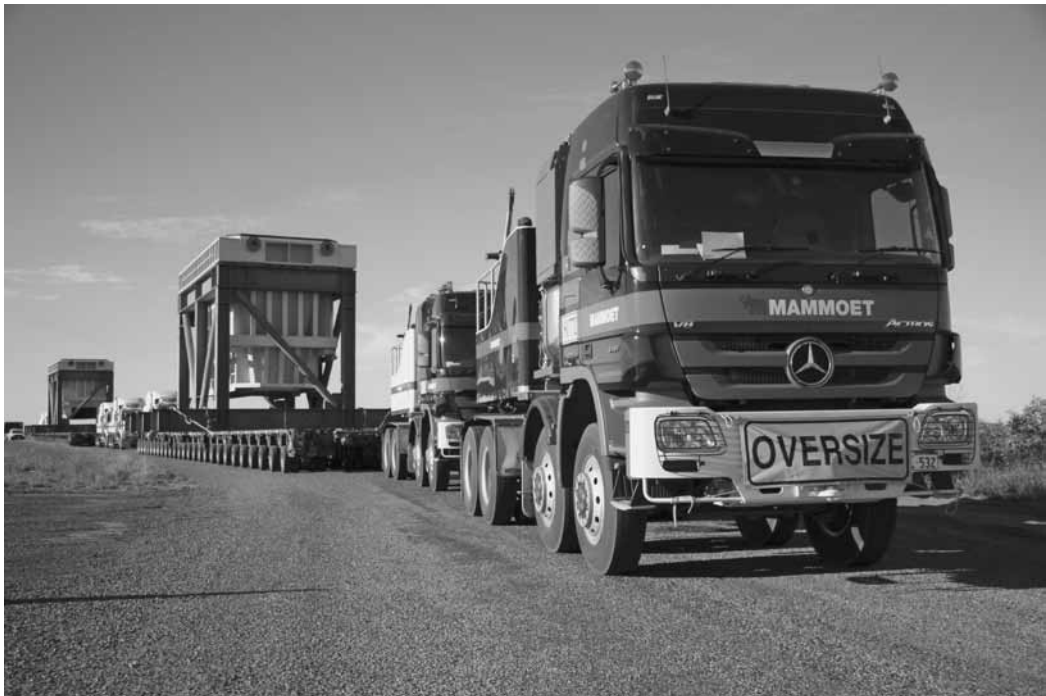
Figure 27.7 Two heavy haulage tractors working in tandem
