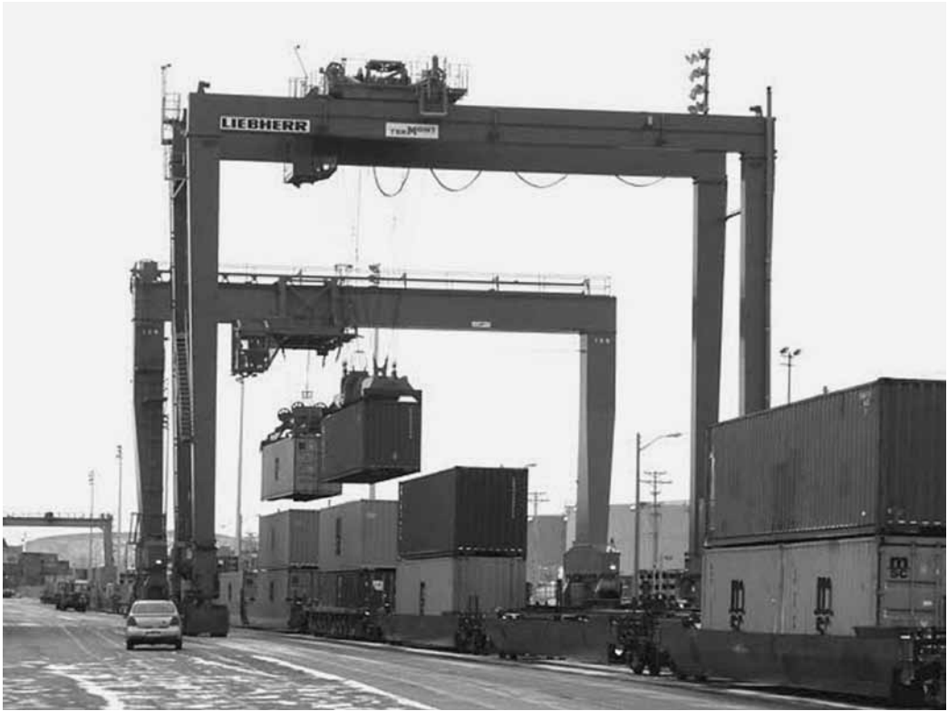
Figure 26.5 Two Gantry cranes loading ISO containers on to railway freight wagons. Note the double-stacked containers as this is in Canada
