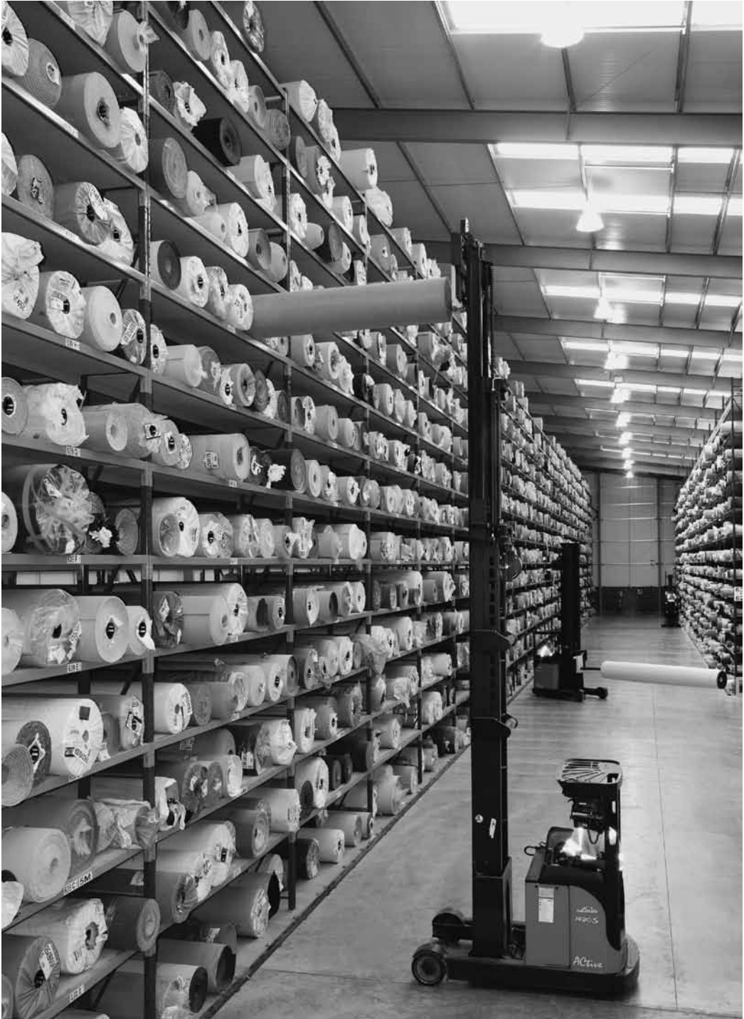
Figure 18.5 Reach truck with boom attachment placing carpet in pigeon-hole racking
