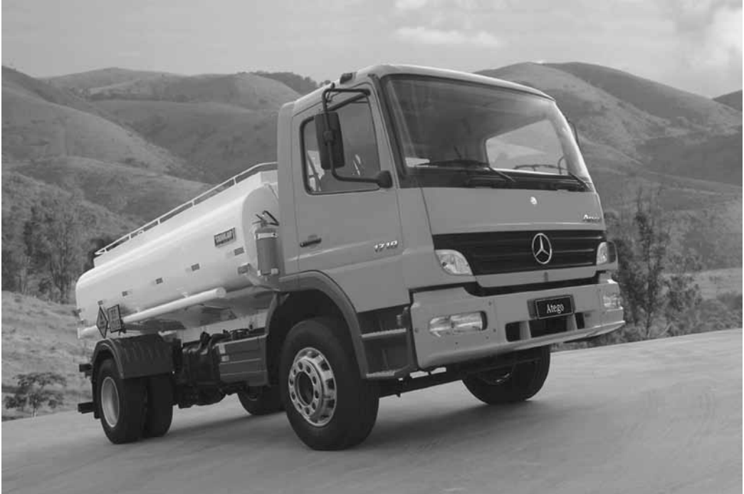
Figure 27.8 A rigid fuel tanker
