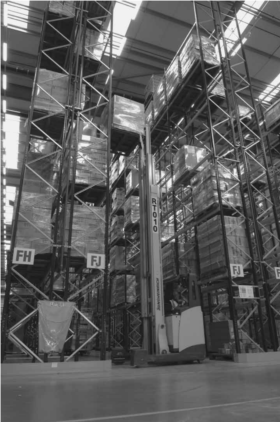
Figure 17.6 Adjustable pallet racking, being served by reach truck, also showing barriers at end of aisle for rack upright protection
