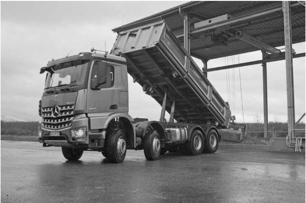
Figure 27.12 An eight-wheel vehicle showing a tipping body
