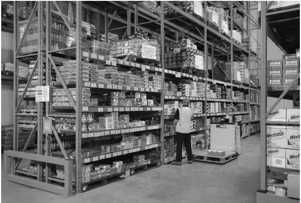
Figure 19.1 Powered pallet truck being used for picking from shelving at the lower level of adjustable pallet racking
