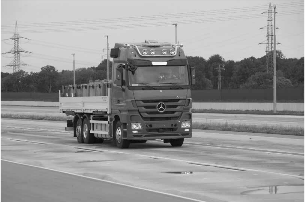
Figure 27.10 A platform or flat-bed rigid vehicle with drop sides
