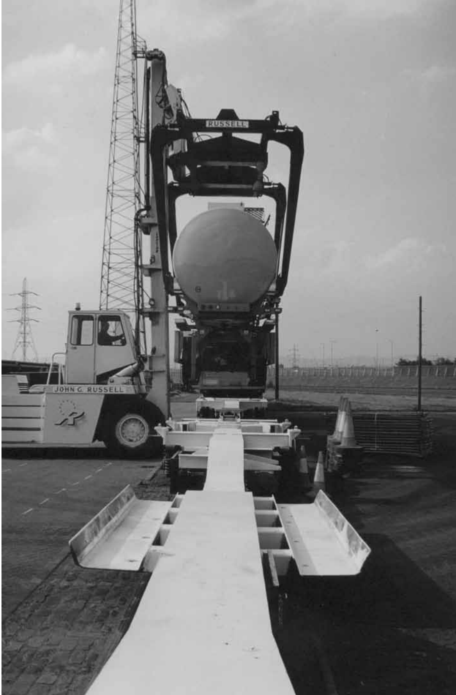
Figure 26.3 Spine wagons being loaded by a reach stacker equipped with a grappeler
