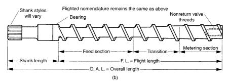
Figure I.2 Components of an injection unit: (a) barrel and (b) screw. (Ref: Barry, C.M.F. and Orroth, S.A., "Processing of Thermoplastics", *Modern Plastics Handbook*, C.A. Harper, ed., McGraw-Hill, New York, 2000)
