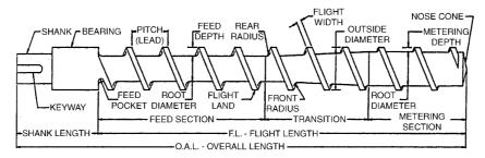
Figure E.5 Nomenclature for sections of an extruder screw. (Ref: Barry, C.M.F. and Orroth, S.A., "Processing of Thermoplastics", *Modern Plastics Handbook*, McGraw-Hill, New York, 2000)
