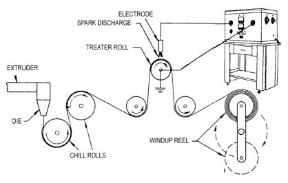
Figure C.7 Basic arrangement for corona surface treatment of plastic film. (Courtesy Lepel High Frequency Laboratories)
