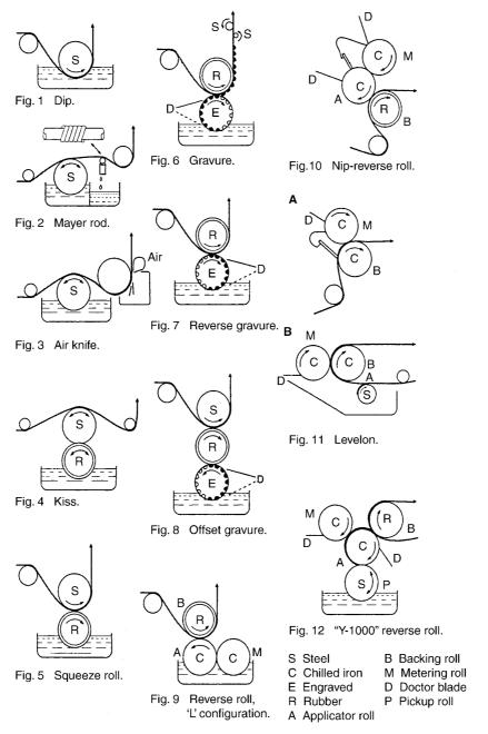
Figure R.4 Schematic representation of the twelve different roll coating processes in common commercial use. (Ref: Somerset Technologies, Inc.)
