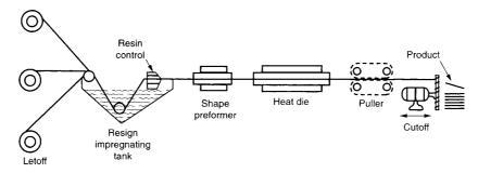
Figure P.24 Pultrusion Process (Ref: Hull, J.L, "Processing of Thermosets", *Modern Plastics Handbook*, 3<sup>rd</sup> ed., C.A. Harper, ed., McGraw-Hill, New York, 1996)
