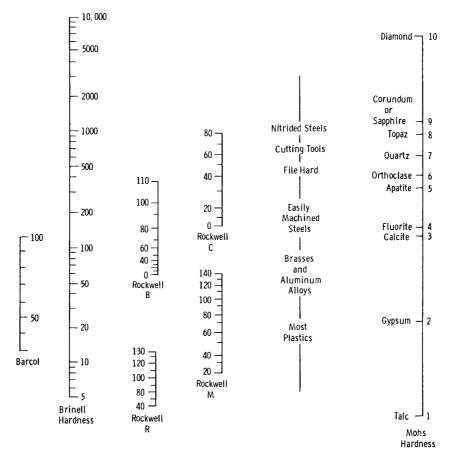
Figure R.3 Comparison of hardness scales. (Ref: Meier, J.F., "Fundamentals of Plastics and Elastomers", Handbook of Plastics, Elastomers, and Composites, 3<sup>rd</sup> ed., C.A. Harper, ed., McGraw-Hill, New York, 1996)
