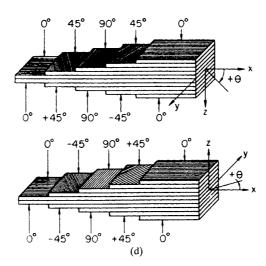
Symmetric laminates with an even number of plies are listed in sequence, starting at one face and stopping at the midpoint. A subscript S following the bracket indicates that only one half of the code is shown. See Figure e.
