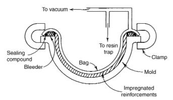
Figure V.1 Vacuum bag molding (Ref: Harper, C.A., "Laminates and Reinforced Plastics Materials and Processes"; *Handbook of Plastics, Elastomers, and Composites*, 3<sup>rd</sup> ed., C.A. Harper, ed., McGraw-Hill, New York. 1998)
