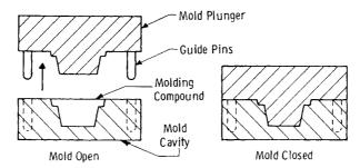
Figure C.4 Simplified illustration of the compression molding process. (Ref: Meier, J.F., "Fundamentals of Plastics and Elastomers", *Handbook of Plastics, Elastomers, and Composites*, 3<sup>rd</sup> ed., C.A. Harper, ed., McGraw-Hill, New York, 1996)
