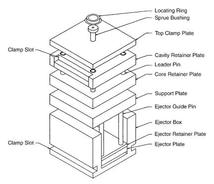
Figure I.4 Generic Parts and Construction of an Injection Mold (Ref: Muccio, E.A., *Plastic Part Technology*, ASM International, Materials Park, OH)
