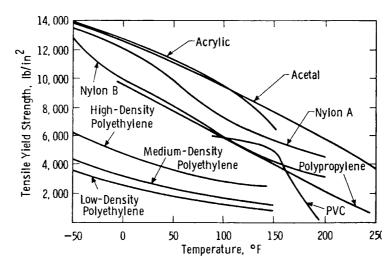
Figure T.4 Tensile yield strength of several thermoplastic materials as a function of temperature. (Ref: Barken H.E., and Javitz, A.E., "Plastics Molding Materials for Structural and Mechanical Applications", *Electrical Manufacturing*, May 1962)
