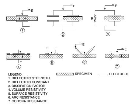
Figure D.1 Schematic illustration of electrical properties. (Ref: Craig, C.L., "Electrical Properties of Plastics" *Plastics Design and Processing*, Lake Publishing Co., Libertyville, Il, February 1962)
