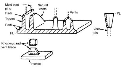
Figure V.2 Ejector pins and vents. (Ref: Hull, J.L.., "Design and Processing of Plastics Parts", *Handbook of Plastics, Elastomers, and Composites*, 3rd ed., McGraw-Hill, New York, 1996)
