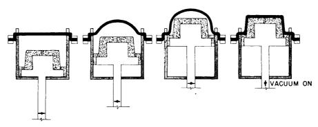
Figure A.7 Air-slip forming process. (Courtesy of Dow Chemical Company)
