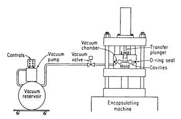
Figure V.3 Schematic diagram showing principle of vacuum venting with transfer molding. (Courtesy Hull Corporation)
