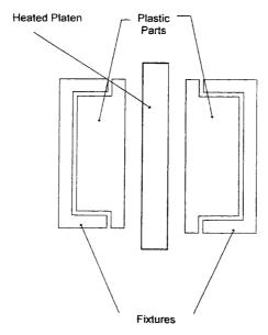
Figure H.2 In direct hot plate welding, two fixtures press components into a hot, movable plate, causing the plastic to melt at the interface. Subsequent removal of the plate, application of pressure on the joint, and cooling time allows the welded joint to form and gain strength.
