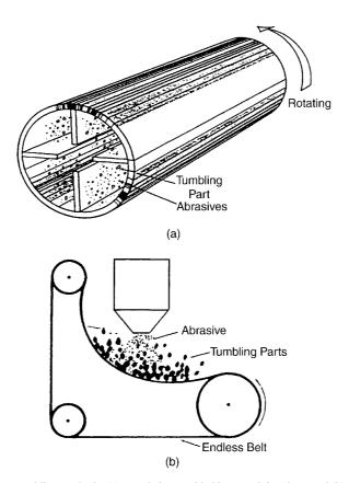
Figure T.9 Two tumbling methods: (a) parts being tumbled in a revolving drum and (b) parts being tumbled on an endless revolving belt. (Ref: Richardson, T.A., "Machining and Finishing" *Modern Industrial Plastics*, Howard W. Sams & Co., New York, 1974)
