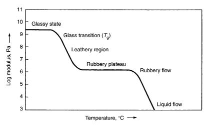
Figure G.2 Relationship between elastic modulus and temperature showing the glass transition region. (Ref: Baker, A.M.M., and Mead, J., "Thermoplastics", *Modern Plastics Handbook*, McGraw-Hill, New York, 2000)
