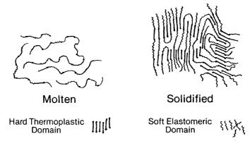
Figure T.7 Morphology of block copolymer thermoplastic elastomers (TPEs). (Ref: Rader, C.P., "Thermoplastic Elastomers", *Handbook of Plastics, Elastomers, and Composites*, 3<sup>rd</sup> ed., C.A. Harper, ed., McGraw-Hill, New York, 1998)
