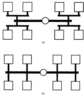
Figure B.1 Runner system: (a) balanced and (b) unbalanced. (Ref: Barry, C.M.F., and Orroth, S.A., "Processing of Thermoplastics", *Modern Plastics Handbook*, C.A. Harper, ed., McGraw-Hill, New York, 2000)
