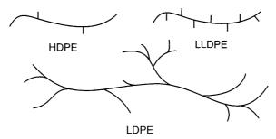
Figure P.12 Chain configurations of polyethylene.
