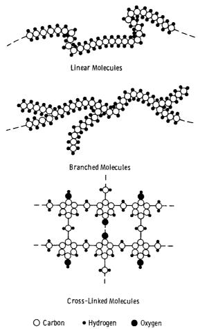
$Figure\ IN.2\quad Some\ possible\ molecular\ structures\ in\ polymers.$
