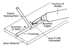
Figure H.5 Hot gas welding process. (Courtesy: Kamweld Plastics, Inc., Norwood, Mass)
