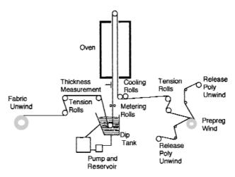
Figure P.22 Schematic of the typical solution prepreg process (Ref: Hull, J.L, "Processing of Thermosets", *Handbook of Plastics, Elastomers, and Composites*, 3<sup>rd</sup> ed., C.A. Harper, ed., McGraw-Hill, New York, 1996)
