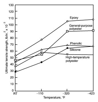
Figure L.3 Cryogenic strength of various laminates. (Landrock, A.H., "Properties of Plastics and Related Materials at Cryogenic Temperatures", Plastics Report No. 20, Picattiny Arsenal, 1975)
