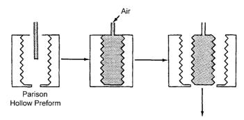
Figure B.3 Schematic depiction of the blow molding process. (Ref: Rader, C.P., "Thermoplastic Elastomers", *Handbook of Plastics, Elastomers and Composites*, 3<sup>rd</sup> ed., C.A. Harper, ed., McGraw-Hill, New York, 1996)
