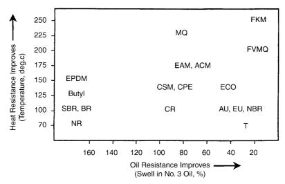
Figure O.1 Heat and oil resistance per ASTM D2000 / SAE J200 schemes. (Ohm, R., and DelVeccio, R.J., "Natural and Synthetic Rubbers", *Handbook of Materials and Plastics Design*, McGraw-Hill, New York. 2001)
