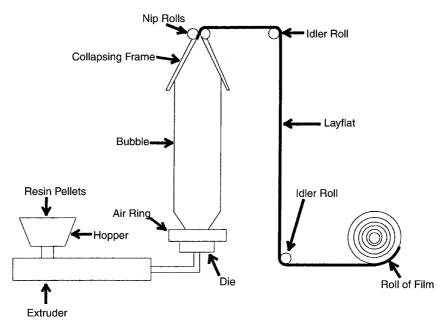
Figure B.4 Schematic of blown film line. (Ref: Barry, C.M.F., and Orroth, S.A., "Processing of Thermoplastics", Modern Plastics Handbook, C.A. Harper, ed., McGraw-Hill, New York, 2000)
