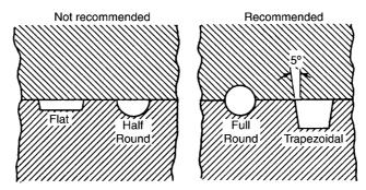
Figure R.6 Runner designs. (Ref: Monsanto Plastics and Resins Co. also Schwartz, S.S. and Goodwin, S.H., *Plastics Materials and Processes*, van Nostrand Reinhold, New York, 1982, p. 876)
