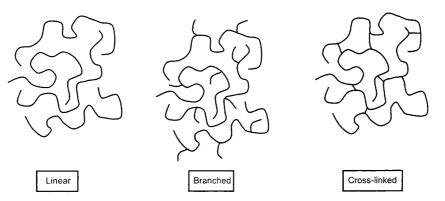
Figure T.6 Linear, branched, and crosslinked polymer structures. (Ref: Baker, A.M.M., and Mead, J., "Thermoplastics", *Modern Plastics Handbook*, C.A. Harper, ed., McGraw-Hill, New York, 2000)
