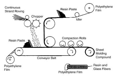
Figure M.5 Sheet molding compound process. (Ref: Harper, C.A., "Thermosets, Reinforced Plastics, and Composites", *Modern Plastics Handbook*, C.A. Harper, ed., McGraw-Hill, New York, 2000)
