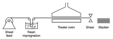
Figure L.1 Horizontal treater for preparing prepreg for laminates. (Ref: Harper, C.A., "Laminates and Reinforced Plastic Materials and Processes", *Handbook of Plastics, Elastomers, and Composites*, 3<sup>rd</sup> ed., C.A. Harper, ed., McGraw-Hill, New York, 1996)
