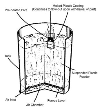
Figure F.4 Illustration of fluidized bed process principle. (Ref: Izzo, C.P., "Protective and Decorative Coatings", *Handbook of Plastics, Elastomers and Composites*, 3<sup>rd</sup> ed., C.A. Harper, ed., McGraw-Hill, New York, 1996)
