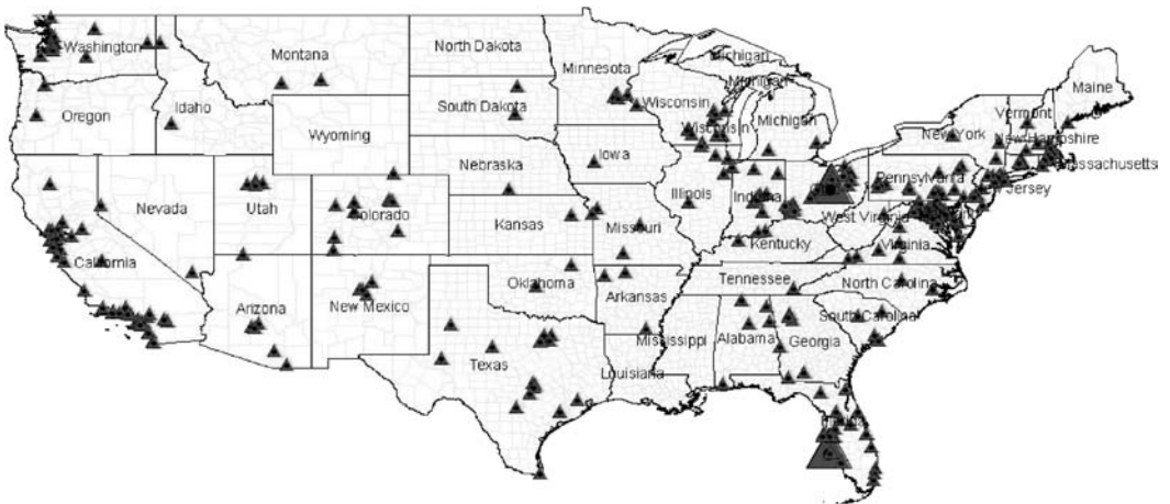
FIGURE 24.1 Plumbing pipe pinhole leak distribution (2000–2004) (small triangles show number of leaks less than 10). (From Lee and Loganathan, Virginia Water Central , Virginia Water Resources Research Center, 2006. With permission.)
