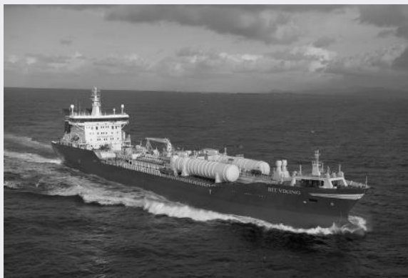
FIGURE 6.13 The Bit Viking owned by Tarbit Shipping after becoming the world's first merchant ship to undergo an LNG conversion. (Courtesy of Wärtsilä.)
