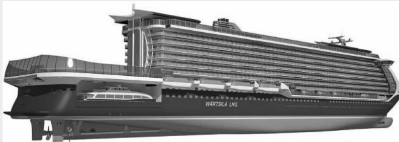
FIGURE 6.9 The concept features a short superstructure with a wide and long hull. (Courtesy of Wärtsilä.)
