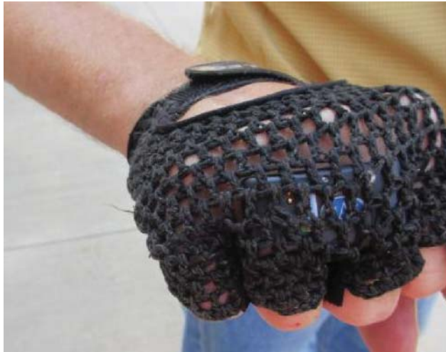
Figure 11.5 HAVSense Sensor Inside Operator's Glove
