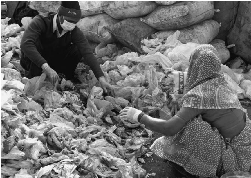
FIGURE 19.1 The plastic bags are selected on colour, cut open, washed and dried.
