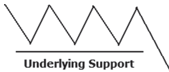
FIGURE 4.3 Test configuration: Underlying support at valleys.
