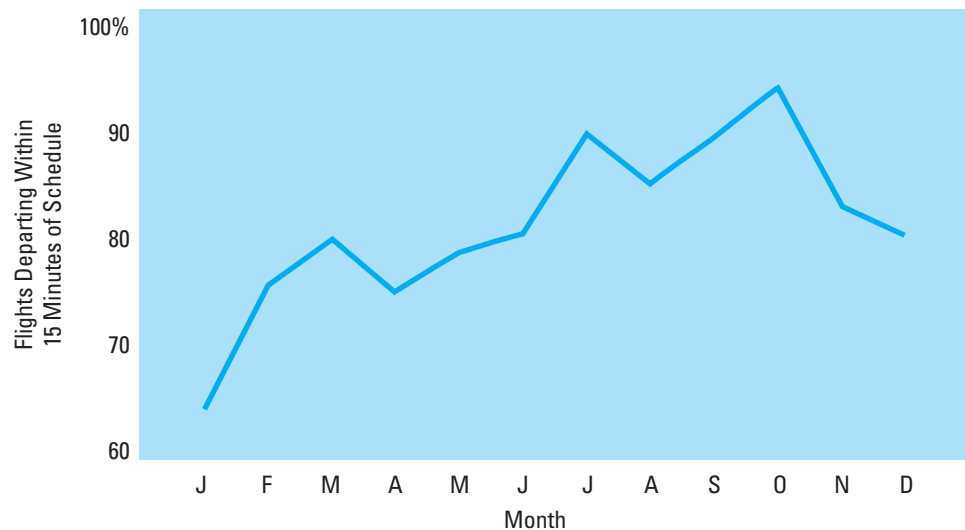
FIGURE 14.6 Control Chart for Departure Delays Showing Percentage of Flights Departing within 15 Minutes of Schedule
