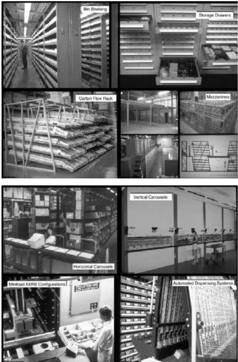
FIGURE 8-26 Small item storage systems.
