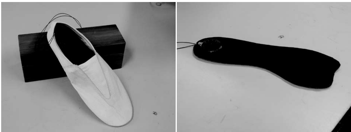
Figure 1. Sensorized shoe for marking the gait cycle
