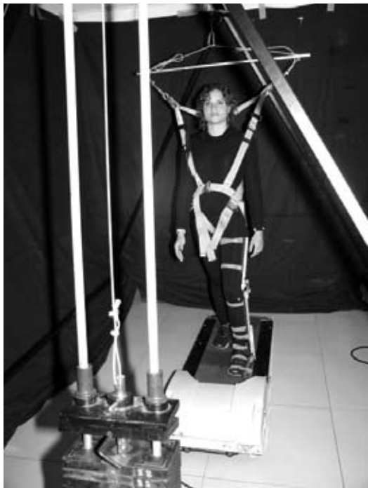
Figure 2. Body suspension device: counterweight system (a); harness used (b); the load cell (c)
