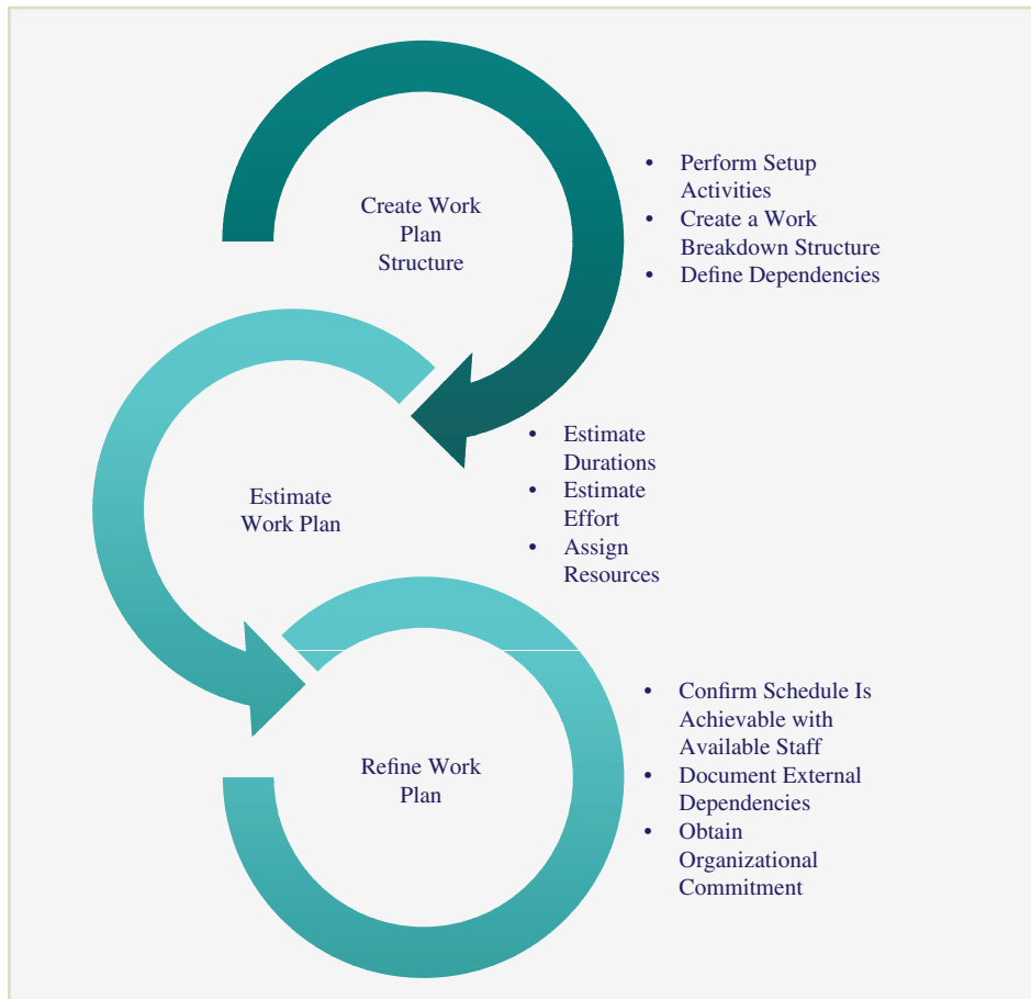
Figure 15–33. Activities required to develop a work plan.
