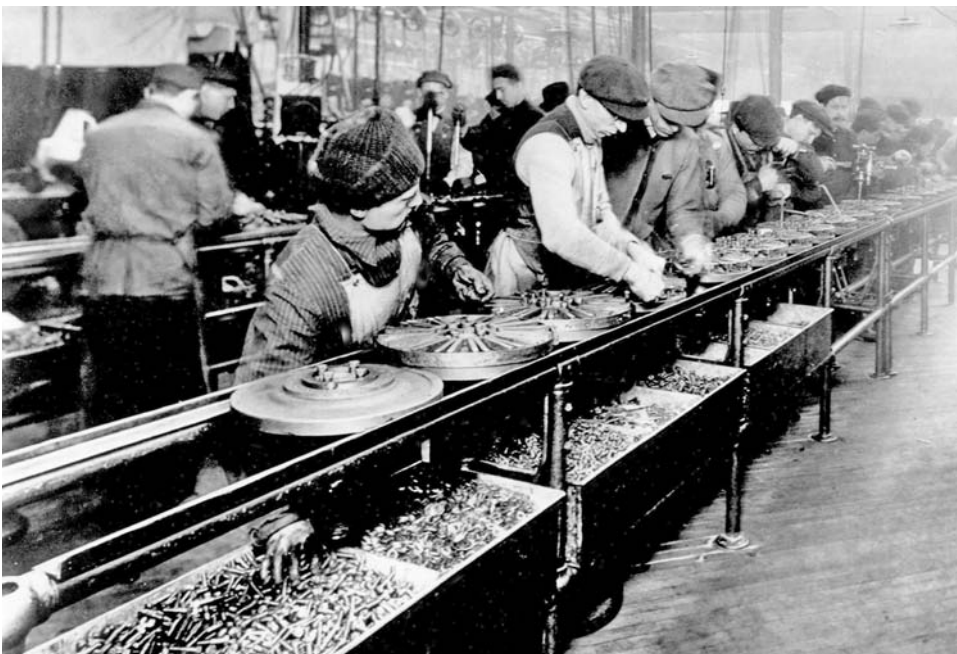
Flywheel assembly line at the Ford Highland Park plant in 1913. (AP/Wide World Photos)
