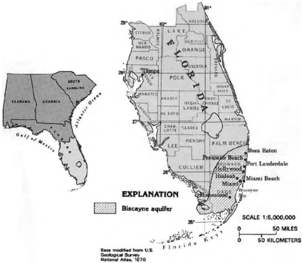
Figure 111.119 The Biscayne aquifer underlies part of four counties in southeastern Florida, and consists predominantly of limestone. (From www.capp.water.usgs.gov . With permission.)
