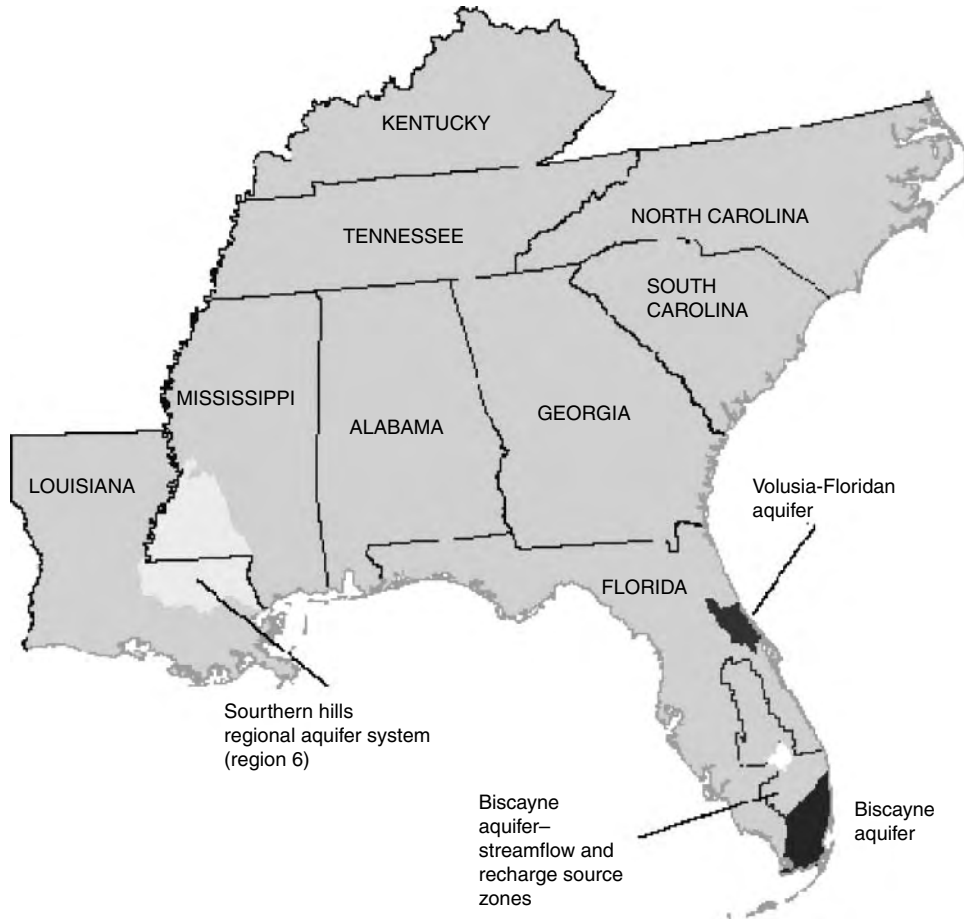
Figure 11I.112 Designated sole source aquifers in EPA Region IV, Alabama, Florida, Georgia, Kentucky, Mississippi, North Carolina, South Carolina, Tennessee. (From www.epa.gov . With permission.)
