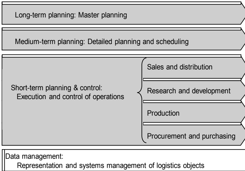
Fig. 5.1.1.1 Business processes in logistics and operations management of an enterprise, structured according to temporal range, with data management.
