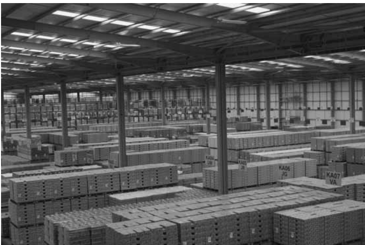
FIGURE 10.2 Example of block stacking (courtesy of Howard Tenens)
