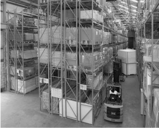
FIGURE 10.3 Double-deep racking (courtesy of Redirack)
