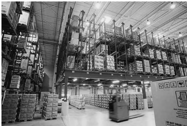
FIGURE 10.9 Shuttle racking above despatch bays (courtesy of Toyota)
