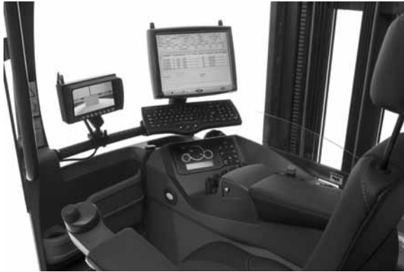
FIGURE 10.18 Internal view of computerized forklift truck (courtesy of Atlet)
