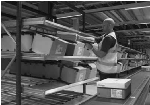
FIGURE 5.16 Carton flow rack (courtesy of Knapp)
