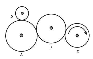
Four rubber wheels, A, B, C and D are touching so that if one moves the others must also move. If wheel C turns in the direction shown, which way will wheel D turn?
