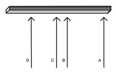
A beam is supported at the points shown by the four supporting arrows, A, B, C and D. Which two arrows could be removed so that the beam remains in the same position?
