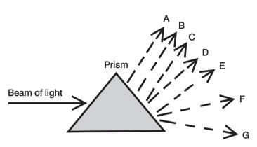
A prism may be used to break up light into its primary colours
