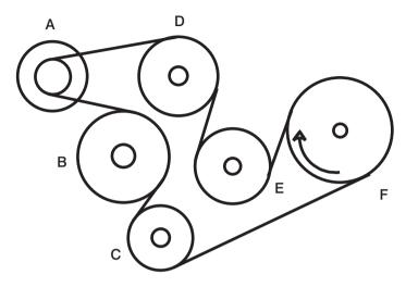
When F turns in the direction shown, which way does A turn?
