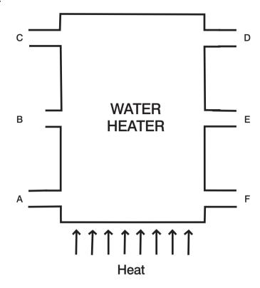
The diagram shows a section through a hot water boiler. As water is heated, the hot water is drawn off through the outlet at D. From which pipe, A, B, C, E, or F should cold water be introduced into the system?
