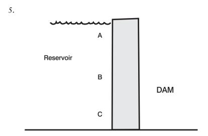
In the design for a new dam shown in section above, at which point does the water exert the greatest pressure?
