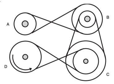
When D turns in the direction shown, which way does A turn?
