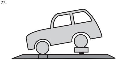
A car, which has no brakes and is not in gear, is easily pushed on to a horizontal ramp. Its rear wheels are then raised as shown. The car is supported only by its free moving wheels.
