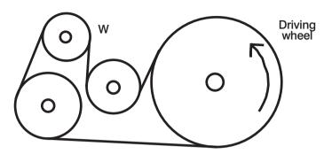
A band passes around all the wheels so that they can all be turned by the driving wheel. When the driving wheel turns in the direction shown, which way does wheel W turn?
