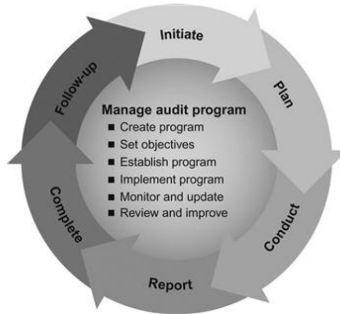
FIGURE 9.3 The ISO auditing process defines six sequential steps in addition to overall audit program management [8,9].
