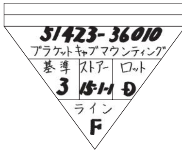
FIGURE 3.7 Triangular kanban for a bracket cab mounting.
