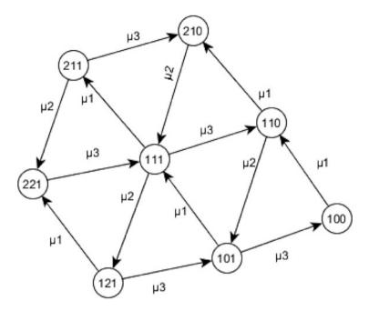
Fig. 9 State transition rate diagram for three station line with no intermediate buffers
