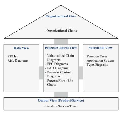
Fig. 2 Methods of the integrated architecture within different views of "ARIS House"
