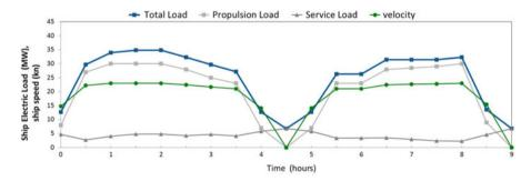
Fig. 2 Ship total load, propulsion load, service load for non-optimized operation
