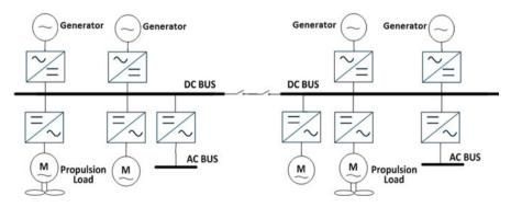
Fig. 1 Generic single-line diagram of AES with dc grid technology
