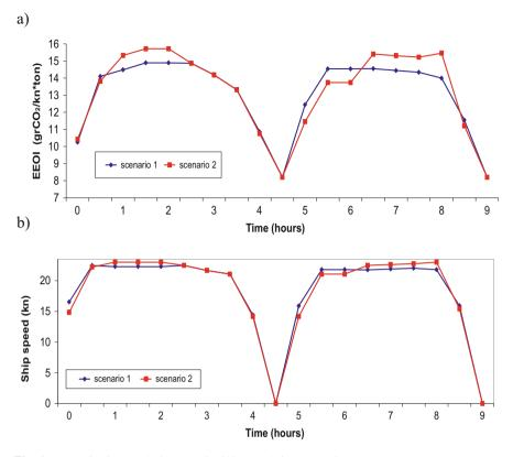
Fig. 4 (a) EEOI time evolution and (b) Ship speed time evolution
