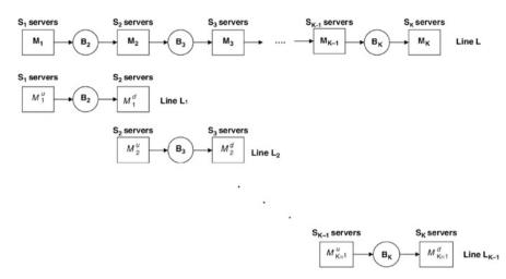
**Fig. 10** Flow line with K parallel-machine work-stations, K-1 intermediate buffers (Line L) and decomposition scheme (Lines L<sub>1</sub>, ..., L<sub>K-1</sub>) (Papadopoulos et al. 2009). In the present work S = 1
