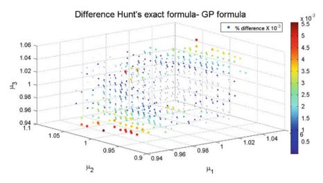
Fig. 4 Difference between Hunt's formula and the proposed GP formula results for three stations in estimation of throughput within the area of the training set. The max % difference is  $5.5 \times 10^{-3}$  for 1000 random points
